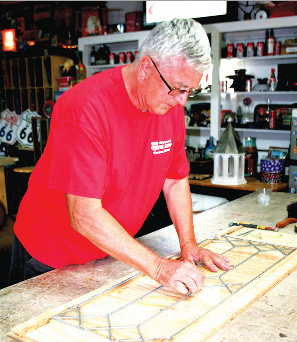
TOM PERKINS of Gardner does repair to a glass window using a “cartoon” scale drawing after cutting pieces to fit. The Paper photo
