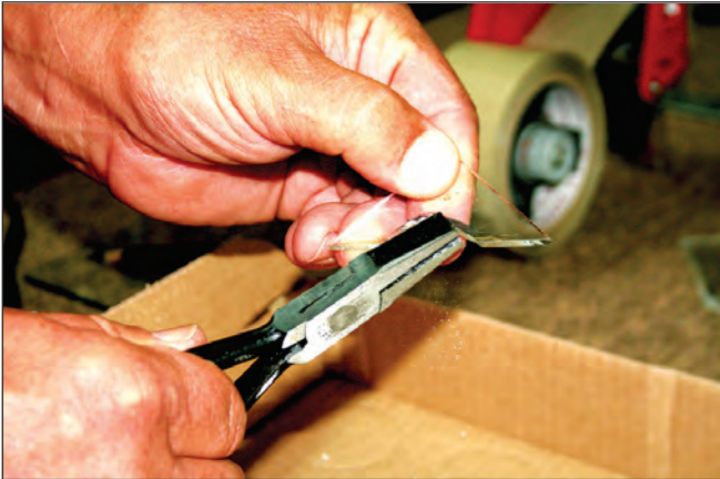
A GROZING pliers is used to nip out shapes in glass.
