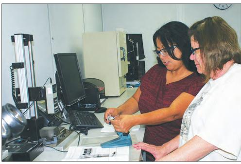
RAQUEL MELENDEZ, (left) quality manager at Peritus Plastics, works with plastics press operator Brenda Clark, of Mazon, checking the measurements of a plastic part on a micrometer in the company lab. The "in-process" checks are performed about twice a shift on parts for quality control. Peritus Plastics, of Mazon, makes about 50 parts for the automotive industry. The Paper photo
