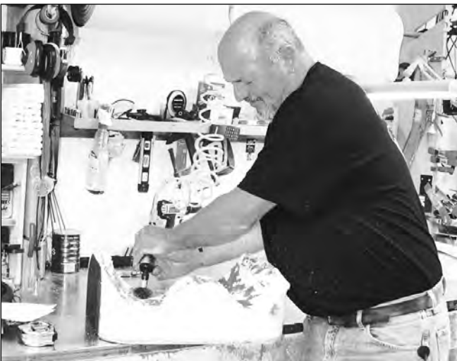
PART OF THE process for building a wheelchair involves carving out a shape for the seat cushion, using flotation foam, as Vern Arnold demonstrates.
