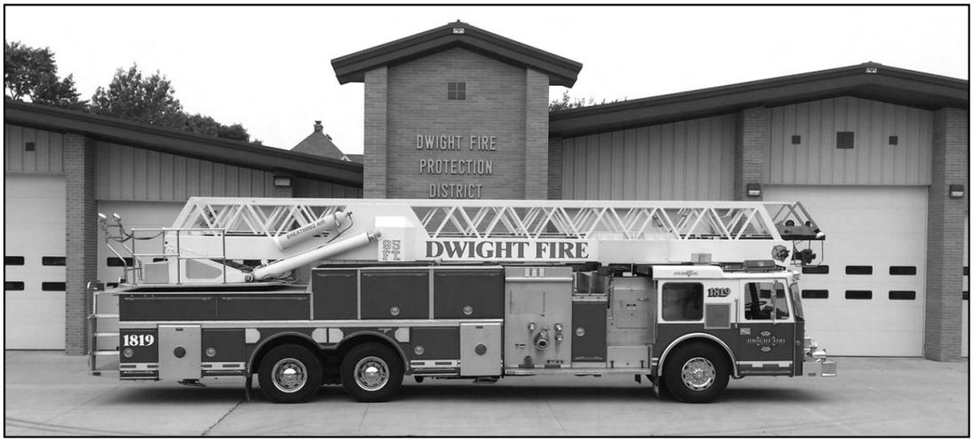
**DWIGHT FIRE PROTECTION DISTRICT** purchased a used Aerial Ladder Truck to join the Dwight Fire fleet. The vehicle is a 1988 Grumman AerialCat that has a 95' aerial ladder equipped with a waterway and pump as well as an entire complement of ground ladders capable of reaching areas up to 35' above grade.
