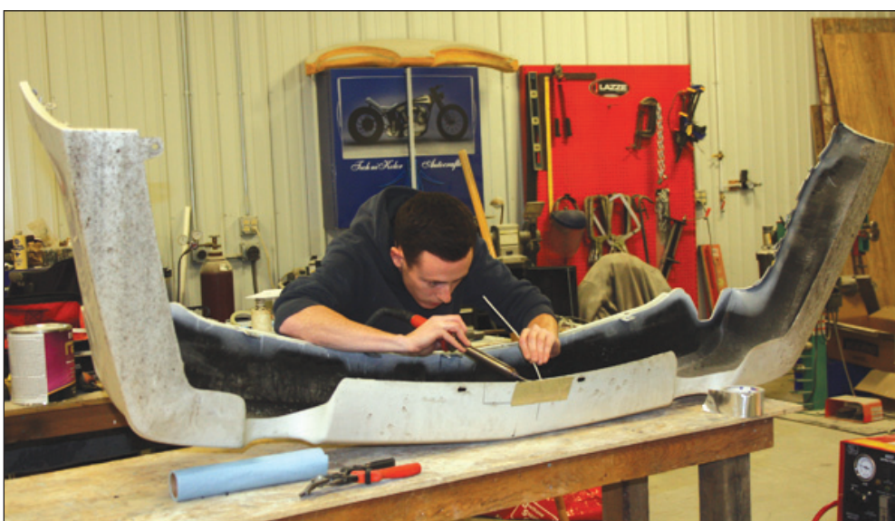
DIRECTLY ABOVE, JOE RUSKIN, Larry's grandson, demonstrates how the newly purchased plastics welder works in the shop at Tech-Ni-Kolor. The welder allows the person using it to reshape the plastic while still maintaining its strength and durability. Pictured top left are Tod Seabert, left, and Larry Seabert, in the shop, with Kooper the dog in the middle.
