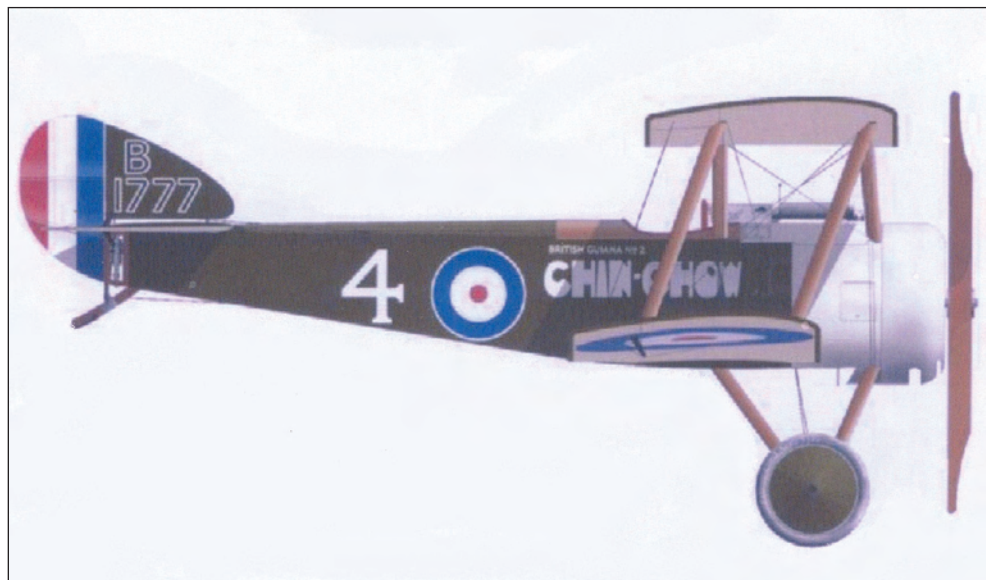
BRITISH SOPWITH PUP. The World War I biplane spans 26'6" and has a fuselage length of 19'. The British markings on the illustration above will appear on the Pup being constructed at Aero Acres. (Log onto Sopwith Pup-You Tube and you can view a Pup in flight.)
