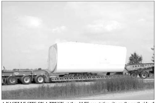
A NACELLE SITS ON A TRUCK at the old FS gas station site on the north side of Dwight. The trucks often wait there for all of the wind turbine parts – the nacelle, several tower sections and three blades - to arrive before traveling through town and to the construction sites in the county. The nacelle houses a generator on top of the tower.
