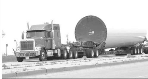
A LARGE TOWER SECTION ARRIVES in Dwight at the Interstate 55 and Route 47 intersection. Once erected, the tower stands about 40 stories high. These tower parts come from Manitowoc, Wisconsin, and from Indonesia, arriving in the United States through the Port of Houston, Texas.
